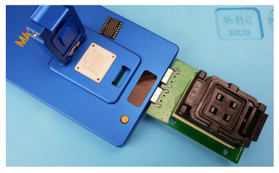
4. Please pay attention to the direction of your hard drive: The first round dot on the left corner of the NAND is its first pin, make sure to align it to the left lower corner of 32+64 Bit socket as the following picture shows:
